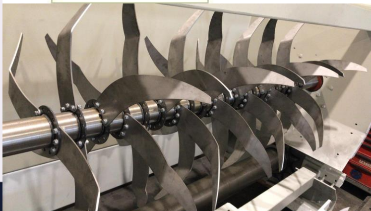
DISCHARGE PADDLE BREAKER
